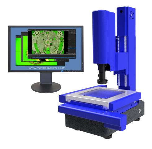
This versatile and automatic workshop measuring machine allows fast and reliable optical measurement on different visual fields. Equipped with the M3 software, this system allows the control of XYZ axis, focus, magnifications and illuminators. Its equipment allows several parts to be measured simultaneously without continuous operator intervention.
